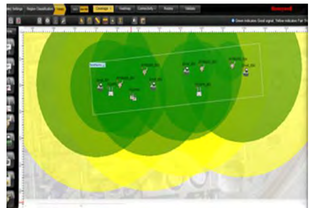
RF Lite provides a graphical display of the wireless network components and field device coverage map.
