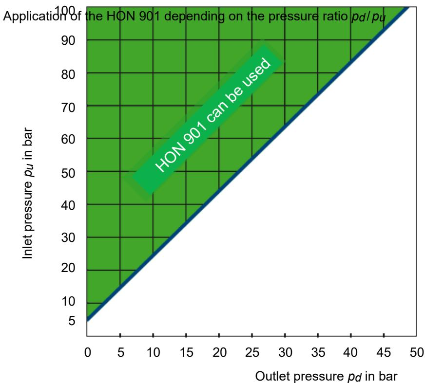
The gas pre-heater HON 901 can be used in the range:  $p_u \geq 2 \cdot p_d + 5$
