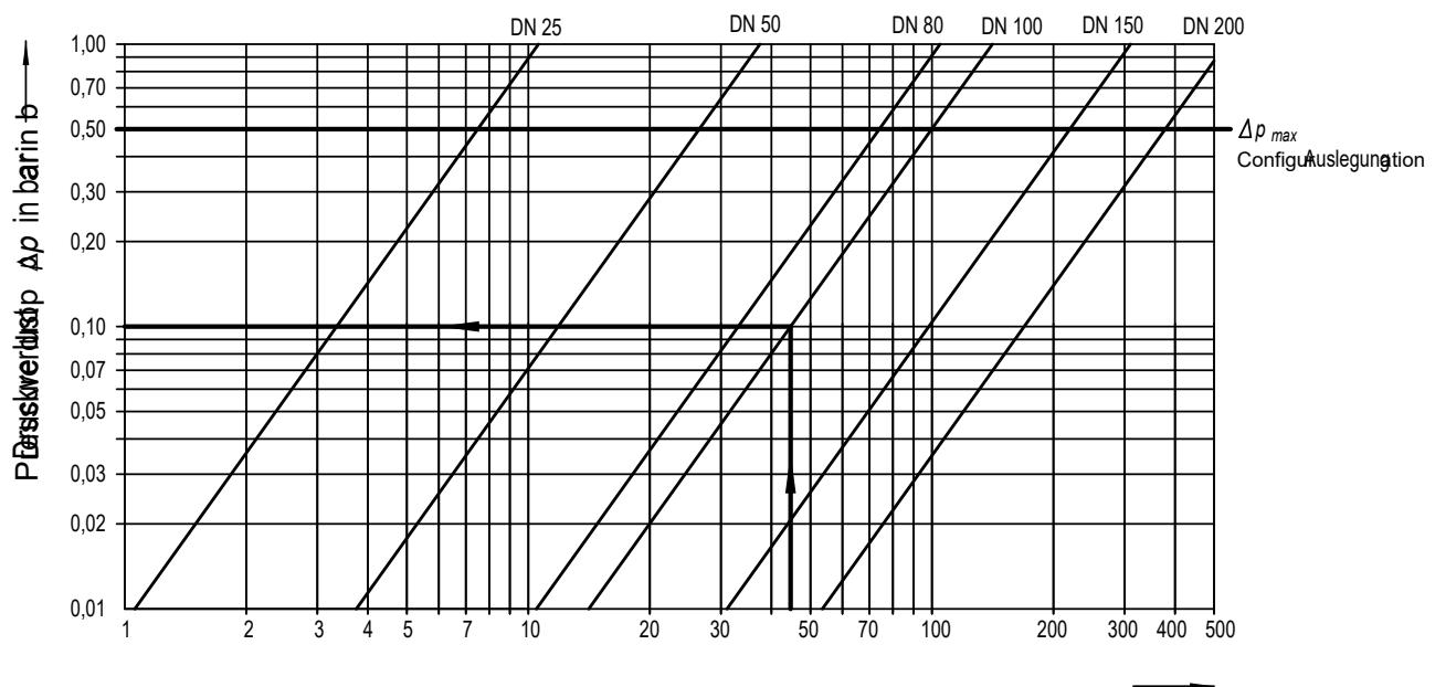
Example: Nominal width DN 100, flow rate  $Q = 45 \text{ m}^3/\text{h} \rightarrow$  pressure loss  $\Delta p = 0.1 \text{ bar}$
