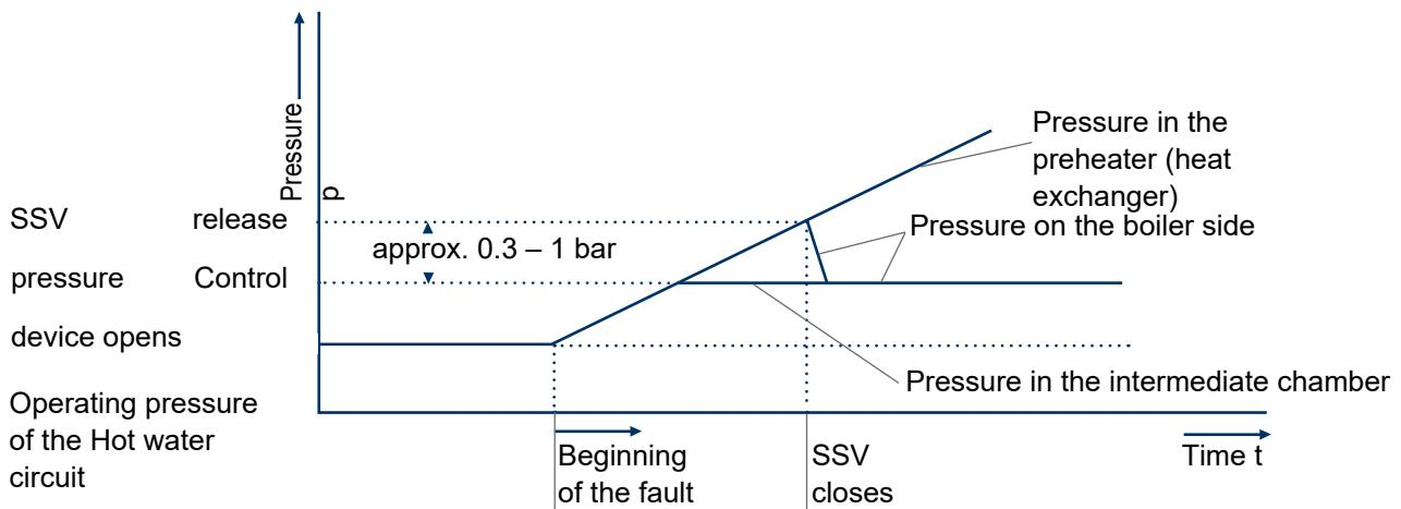
The safety shut-off device (SSV) then opens again if the pressure in the heat exchanger (above the valve plate) is brought to a value below the release pressure of the control device (SSV release pressure minus 0.3 to 1 bar). The remote indication is available in two different versions depending on the temperature in the hot water circuit; it cannot be retrofitted up to DN 200.
