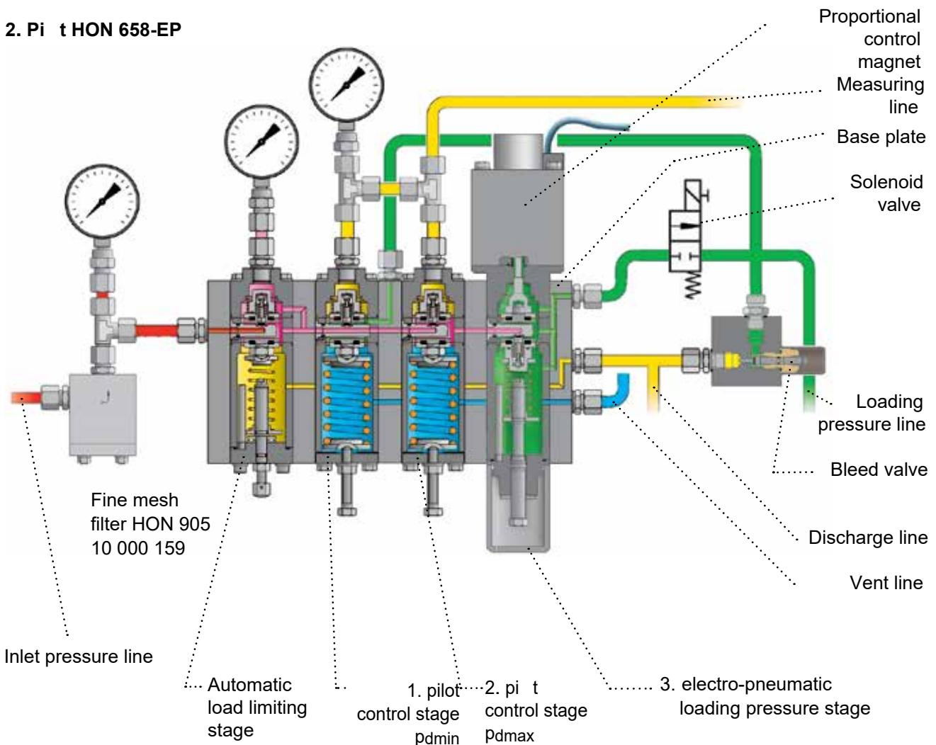
The pneumatic pilot control stages automatically monitor the configured limit values. As soon as the equipment gets close to these limit values during operation, the pilot control stages are activated and keep the outlet pressure constant. Transition between the electro-pneumatic loading pressure stage controlled by the electronic controller and pressure limiting by the pilot control stages is effected independently and without jolts in both directions.
