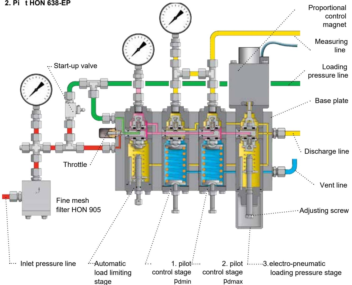
The pneumatic pilot control stages  $p_{d\min}$  and  $p_{d\max}$  automatically monitor the configured limit values. As soon as the equipment gets close to these limit values during operation, the pilot control stages are activated and keep the outlet pressure constant. Transition between the electro-pneumatic loading pressure stage controlled by the electronic controller and pressure limiting by the pilot control stages is effected independently and without jolts in both directions.
