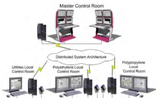
DSA with Master Control Room at a Polymers Complex
