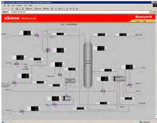
Experion eServer Standard Access provides read-only, real-time information updates through the browser-independent web based environment on the user's desktop or tablet. Users can access the same Experion custom graphics as provided to the control room. The browser refresh button can be used to obtain refreshed Experion data, and eServer Standard Access can be made available to a large number of clients.
