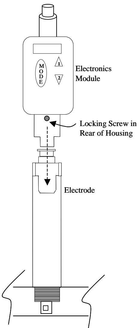
Figure 3—Integral Mounting
