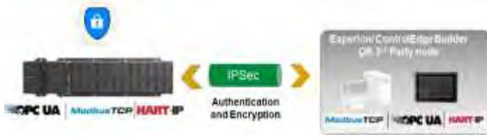
Figure 6. PLC Communication Secured with IPsec
